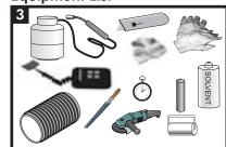
Propane tank, hose, torch & regulator Induction coil & generator Appropriate tools for surface abrasion (grinder, rasp, paper) Knife, roller, rags & approved solvent cleanser Digital thermometer with suitable probe Standard safety equipment; gloves, goggles, hard hat, etc.
