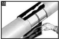
Remove the remaining release liner.
