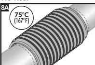
r propane torch(es), pre-heat the joint area to > 75°C (167°F). When heating with
