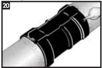
Test sleeve adhesion by gently pressing the sleeve edge with a gloved finger. The sleeve is well bonded when the adhesive and coating remain intimately contacted. If required to improve bonding, additional heat should be applied to the sleeve
