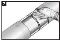
Wipe clean or air blast the steel and pipe coating to remove foreign contaminants. Conduct salt contamination, surface cleanliness and surface profile checks in accordance with client procedures, requirements and frequency.
