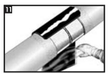
Remove the remaining release liner.
