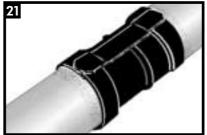
Visually inspect the installed sleeve for the following: Sleeve is in full contact with the steel joint.
